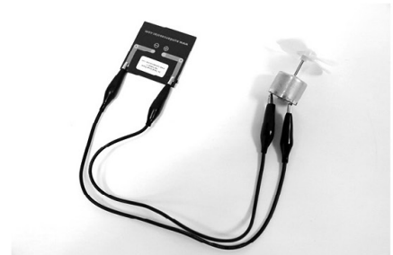
Solar Cell System
