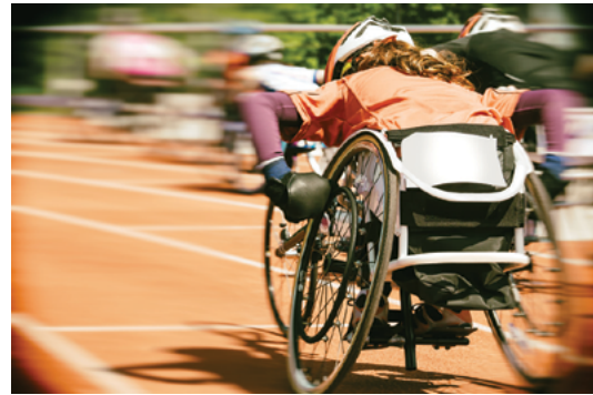
Wheelchairs built for racing need to be light. The less mass the chairs have, the farther they can go on a single push.
