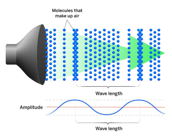
Sound waves occur when an object, like part of a speaker, vibrates. The vibration pushes nearby molecules into the molecules next to them, and those molecules are pushed into the molecules next to them, and so on, forming a wave that moves away from the speaker. When molecules are pushed into the molecules next to them, it's called compression.
